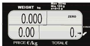
This arrow indicates that the scale AC adaptor is connected to the 220 VCA
