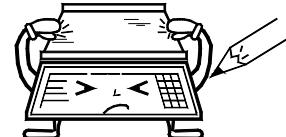
4. Use a 220 v ac outlet exclusive for the scale avoiding overload or voltage variations.
