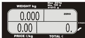
If not, see reference to zero section. Then place the product to be weighed on the plate and you will see the weight in the corresponding indicator.
