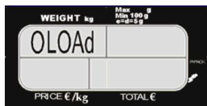
This message indicates that a weight that exceeds the maximum capacity has been placed on the scale. To correct it simply, remove the over weight.
