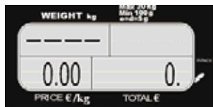
This message indicates a negative weight, this could happen if you lift or remove the scales plate to correct this put the plate back in its place and press the
