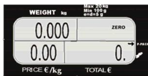
This arrow indicates that the scale is working under the "FIXED PRICE" mode.
